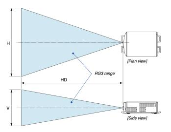
Note: If lens shift is utilized, please consider the shift of projected image according the volume of lens shift.
