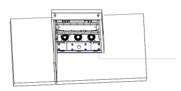
Place the kisok on the foundation, Use nuts corresponding to M12/M16 bolts for fixation, ensuring proper tightening.
