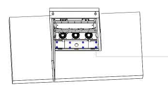
Place the kisok on the foundation, then tighten the nuts to secure.
